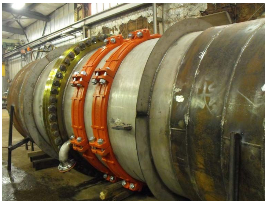
Testing of the 72" (1800 mm) Shurjoint Ring Joint Coupling Assembly
