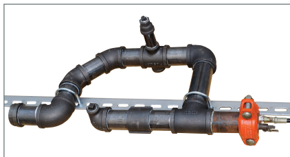
Burst pressure testing of DI threaded fittings (2’)
