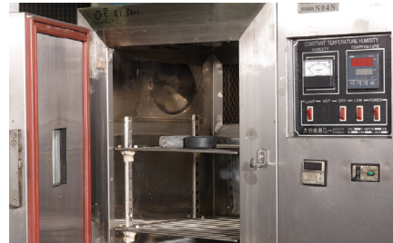
Laboratory high temperature oven testing
