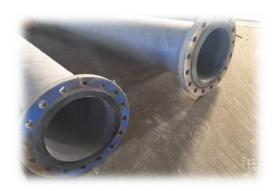
A typical connection that can still be found in the mining industry is the flange connections. These are still commonly used to connect pumps and flanged pipe, but they do have some disadvantages such as:
