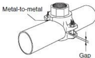
It is normal to see bolt pad gaps, though they should be equal on both sides of the mechanical tee.
