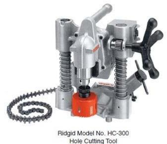
**Hole Size:** The hole sizes are dictated by the branch size of the mechanical tee. Refer to each product data sheet, F-01 (#7721), F-02 (#7722), F-07 (#M21), F-08 (#M22), F-03 (#723), K-10 (#SS-723), and L-17 (#C723).
