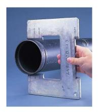
The Shurjoint groove gauge is a handy and helpful tool in checking both the groove diameter and pipe OD.
