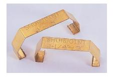
Couplings with rubber gaskets are likely to function as an insulator. Where electrical continuity is required, the Shurjoint continuity clip will restore electrical continuity to the system. The electrical continuity clip satisfies IEE Wiring Regulations.
